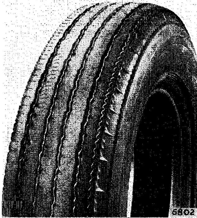
Fig. 3. Fin and feather wear due to extreme wheel misalignment.
