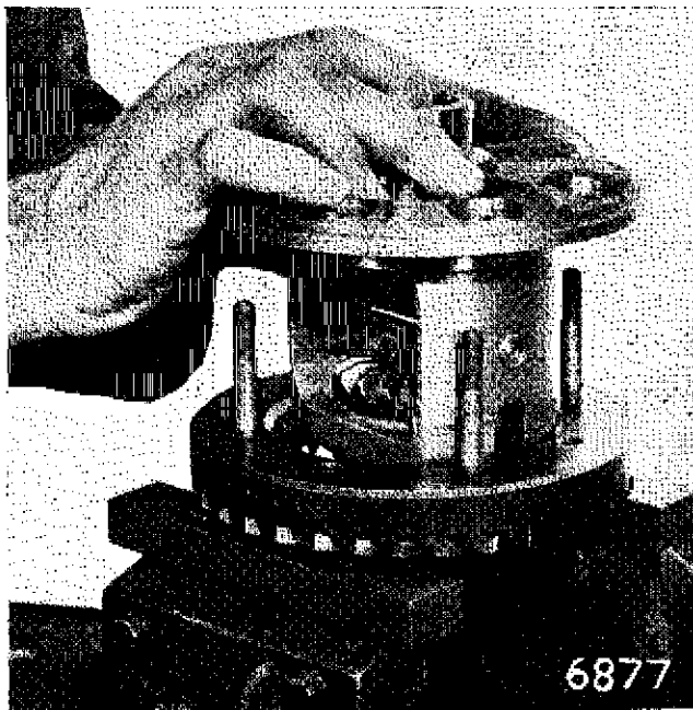
Fig. 40. Fit crown wheel to case
